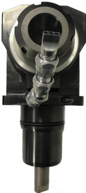
HECTO system mounted in rotary tool holder. Straight nozzle ID:3 mm x 3 & L:20 mm
