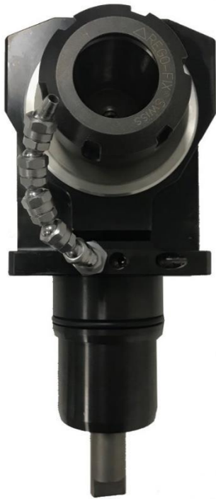
DECA system mounted in rotary tool holder. Straight nozzle ID:3 mm & L:10 mm
