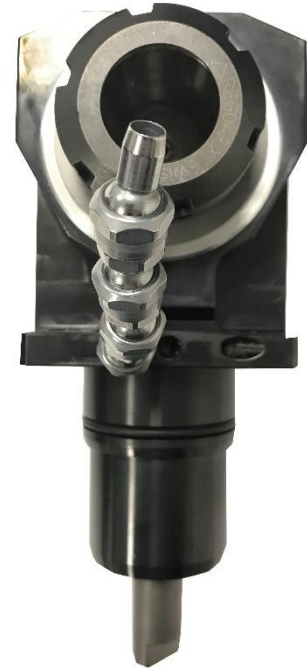
HECTO system mounted in rotary tool holder. Straight nozzle ID:6 mm & L:16 mm
