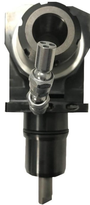
HECTO system mounted in rotary tool holder. Straight nozzle coaxial ID:3.4 x 3 & L=20 mm
