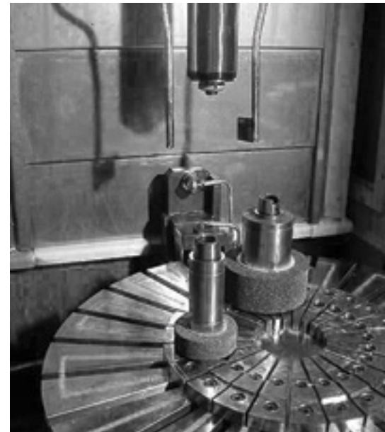
Grinding flange with HSK holder. Magnet adaptors to avoid set-up change for ID and OD grinding.
