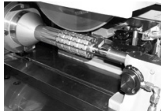
Deep grooves of hydraulic pump rotors are preferably machined with CBN wheels in creep-feed mode
