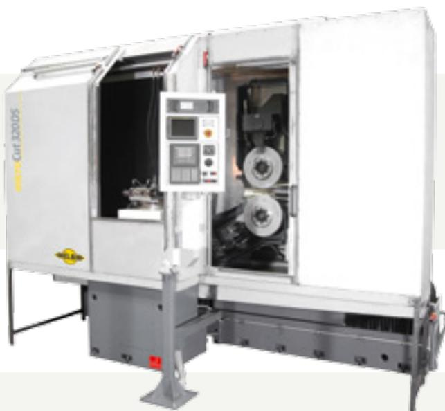
Profile dressing of the grinding wheel can be performed on the table or with headmounted roll dressing units. Head-mounted dressing units can be used intermittently or continuously. To accommodate for the offset between two profiles the position of the upper dressing unit can be adjusted in the cross direction via CNC controls. This machine is commonly used to grind the fir tree profile on turbine vanes.
