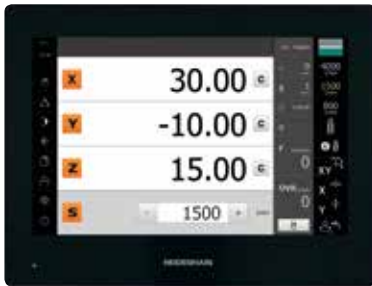
Simple, rapid spindle speed adjustment via touch screen, enter and save values directly on the display.
