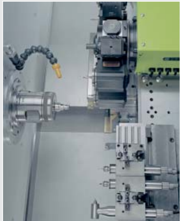
Turrets in the star design size VDI 25 with 12-fold individual plate drive and additional linear tool built on with 3 high-frequency spindles.
