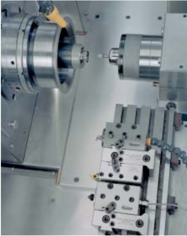
Linear tool design with additional grinding spindle
