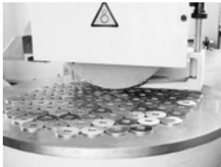
Economical grinding of a table load of small work pieces. In contrast to reciprocating machines the grinding wheel stays in contact with the work pieces. Time savings of up to 25% can be achieved.
