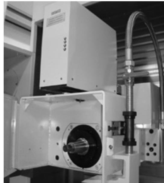
Head-mounted straight-line dressing unit. Best method to dress wheel circumference. No interfering contours no matter how high the work piece.
